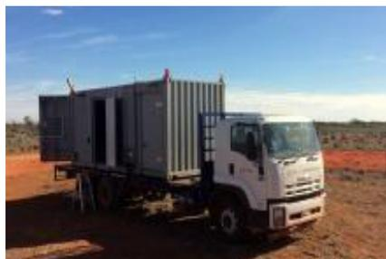
The first Typhoon was commissioned in 2012 and is housed in a customised 20' (6m) ocean container, together with a 230kVA diesel generator for power.
